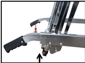
Press button on top of the handle to change horizontal position of front extension handles.
