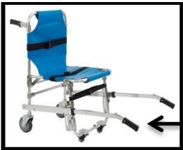
The handles in front of the stair chair extend for easy transportation. The extension handles have 2 locking positions. Lock handles beneath the chair seat, then pull up and adjust. Release button to change position.
